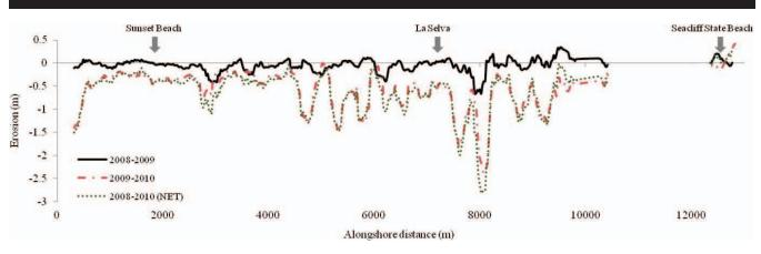
Figure 6. Northern study area plot of shoreline recession with a 100 m running average at 10 m elevation (NAVD88). *X* axis represents alongshore distance (m) starting from Sunset Beach and ending at Seacliff State Beach. *Y* axis represents shoreline recession (m).
