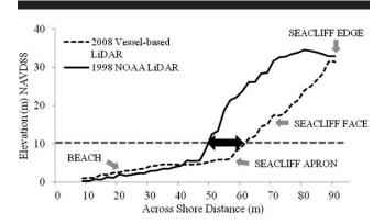
Figure 2. Shore-normal profiles of 1998 and 2008 LIDAR digital elevation models showing an example of shoreline recession measurement with the erosion reference feature being the position of the seacliff face at 10 m elevation NAVD88 (grey dashed line).
