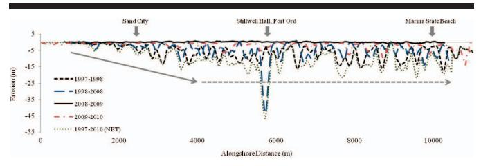
Figure 4. Southern study area plot of shoreline recession with a 100 m running average at 10 m elevation (NAVD88). *X* axis represents alongshore distance (m) starting in Sand City and ending at Marina Sate Beach. *Y* axis represents shoreline recession (m). The solid line depicts a trend of increasing erosion magnitude alongshore, whereas the dashed line depicts signs of shoreline averaging found along this stretch of coastline.
