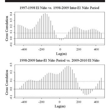
Figure 8. Cross-correlations between consecutive El Niño and inter-El Niño period hot spot erosion for Southern Monterey Bay. The most significant cross correlation values were found at a spatial lag of -160 m (top) and 100 m (bottom), indicating mean alongshore shifts in hot spot locations between periods. Horizontal dashed lines represent 95% confidence levels. Anomalously high shoreline recession values at Stillwell Hall were omitted.
