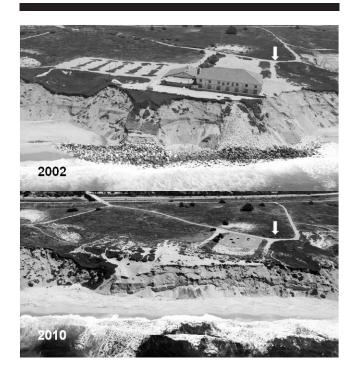
Figure 11. Aerial photographs of Stillwell Hall at Fort Ord captured in 2002 and 2010. [Photos copyright (c) 2010, Adelman and Adelman (2010), Kenneth and Gabrielle Adelman, California Coastal Records Project, www. californiacoastline.org.] This location is a good example of passive erosion fronting coastal armoring, which can be recovered with armor removal.
