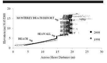
Figure 3. Shore-normal profiles of 2008 vessel-based LIDAR and 1998 aerial LIDAR to assess intersurvey precision. Location: Monterey Bay Beach Resort.
