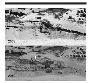
Figure 5. Aerial photographs of the Marina launch ramp at Marina State Beach captured in 2008 and 2010. Shoreline recession was measured at up to 8 m in this area. [Photos copyright (c) 2010, Adelman and Adelman (2010), Kenneth and Gabrielle Adelman, California Coastal Records Project, www. californiacoastline.org.] Resistant horizontal band in seacliff is a paleosol within the Quaternary Aromas Red Sandstone depicted with the horizontal black arrows.
