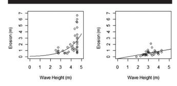
Figure 10. Bluff erosion (m) plotted against average wave height (m) for southern Monterey Bay (left, N=46) and northern Monterey Bay (right, N=34) during the 2009–10 El Niño period with their respective exponential (left) and linear (right) regression lines.
