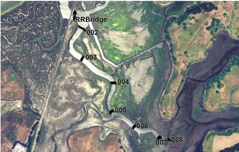
Figure 4. The 2006 eight cross-sectional lines and survey area of Parsons Slough. These were modeled after the Sampey 2003 survey.
