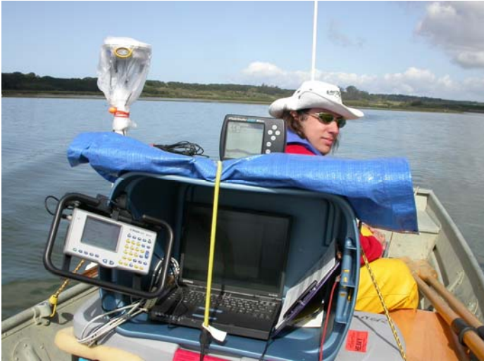
Figure 5. Single beam survey set-up including GPS receiver, ecosounder and data acquisition computer running Hypack® software.
