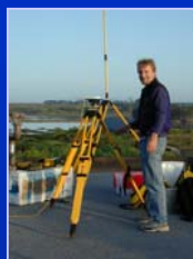
CSUMB student, Jim Brantner establishes a GPS base station for reliable differential corrections of acoustic mapping data.
