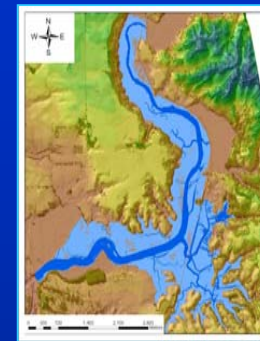
Figure 2. Aerial extent of Elkhorn Slough tidal prism showing MLLW (Low Low Water) and MHW (Mean High Water) contours as calculated from merged DEM.
