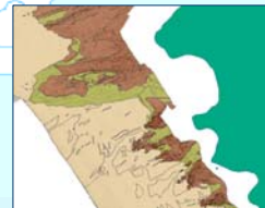
In ArcGIS®, multibeam bathymetry DEMs and the video imagery were used to trace polygons outlining different types of substrate (rocky substrate, degraded (sediment dusted) rocky substrate, and sediment).
