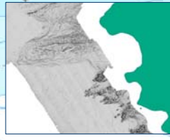
Multibeam bathymetry (and sidescan sonar) data was collected using a Reson 8101 sonar system from aboard the Seafloor Mapping Lab's 27ft vessel R/V MacGinitie
