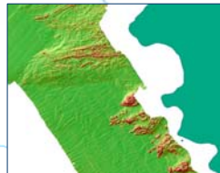
Automated rugosity analysis was also applied to the 2m grid as a way of delineating rocky versus sedimentary habitats. This algorithm calculates a planar area to surface area ratio for each cell in a DEM grid using the elevation of the cell and its eight neighbors. Flat areas (green) will result in ratios near 1, while bumpy, high relief areas (red) will exhibit higher rugosity values. ArcView® 3.x extension Surface Areas and Ratios from Elevation Grids (surfgrids.avx, Jenness Enterprises- www.jennessent.com)
