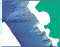
Bathymetric data were post-processed using CARIS HIPS hydrographic data cleaning system software. Corrected data were exported as decimated x,y,z ASCII text files (shoal biased) with 2m spacing and used in additional programs to generate a 2m bathymetry grid.
