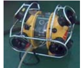
Hyal9 ROV with digital video recorder
